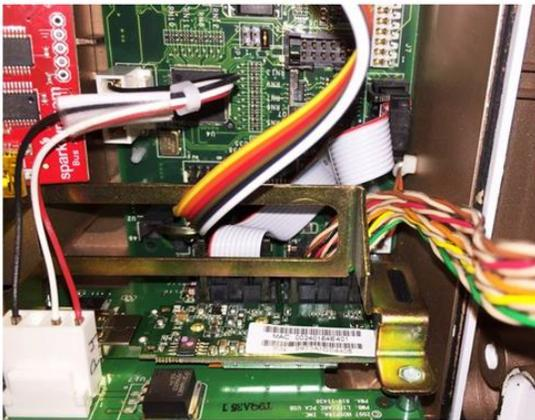
Hospira's drug infusion pumps include a serial cable (the wide grayish-white cable with the single red stripe on one edge) that connects the communications module to the main pump board. © BILLY RIOS
